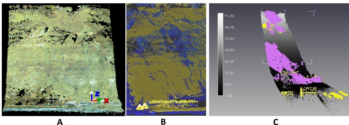
**Fig. 2.** Visualization of the cliff from the Gdansk Bay side. **A:** natural colours, **B:** differences in the cliff's geometry with areas comparison **C:** differences in the cliff's geometry greater than 0.10m
